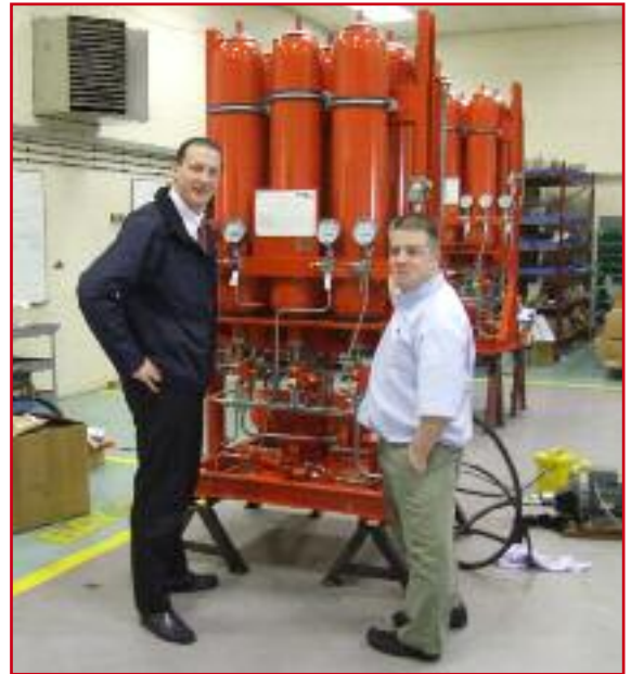
(Above) One of IPU's Hydraulic Starting units featuring Pirtek hoses and some of the many gauges supplied by Oldbury.
